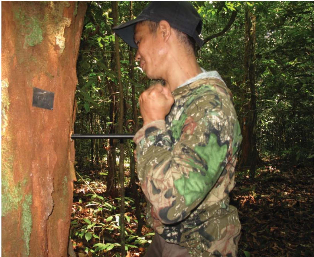
Supi, a member of the field staff at Cabang Panti in West Kalimantan, Indonesia, takes an increment core sample from a Dipterocarpus species. Photo: E. Dormontt/University of Adelaide
